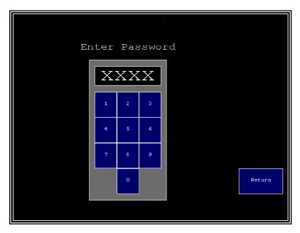
• Enter the four-digit password (including any leading zeros). For example, if the password is 1, enter **0001**.
